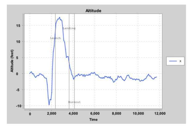
This is an example of the kind of graph that is generated. This graph is from me throwing STARLIGHT about twenty feet into the air. Obviously, the graph will be much smoother when it's over a longer period of time and the rocket flies higher. Graphs will be similar for STARLIGHT MINI, as it uses the same pressure sensor. In this graph, burnout is detected late because the board was in free fall the entire time, with no forces being applied.
