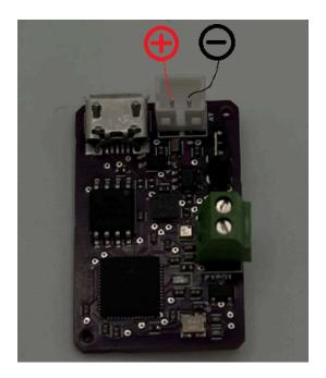
It's recommended to power STARLIGHT MINI with a 1s LiPo battery. STARLIGHT MINI can be powered with anywhere from 2.8 to 6V.
